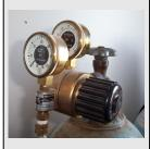
Before a regulator valve is connected, the valve should be opened slightly and closed immediately to clear the valve of dust or dirt. Stand to the side when doing this.
