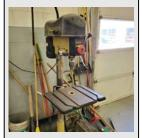
This drill press should have a shield to protect operators in case the chuck key is left in the chuck prior to operation.
