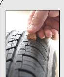
Check tires for proper tread wear, tire pressure, or damage
